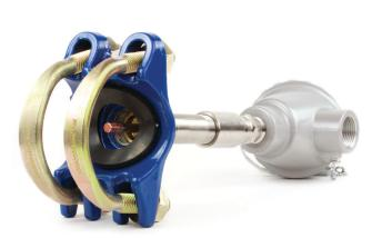
This design incorporates a Burns spring loaded Series 200L RTD and a saddle clamp. A copper tip on the sensor further improves response time and accuracy.
