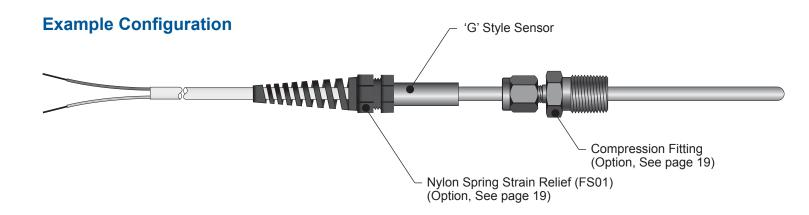
NOTE 1: For sensor sheath lengths 'L' greater than 200 inches contact Burns Customer Service.
